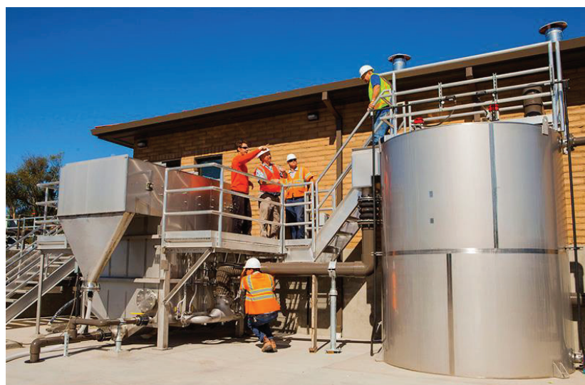
Suspended Air® Flotation System, mixing tank on the right and flotation cell on the left.
