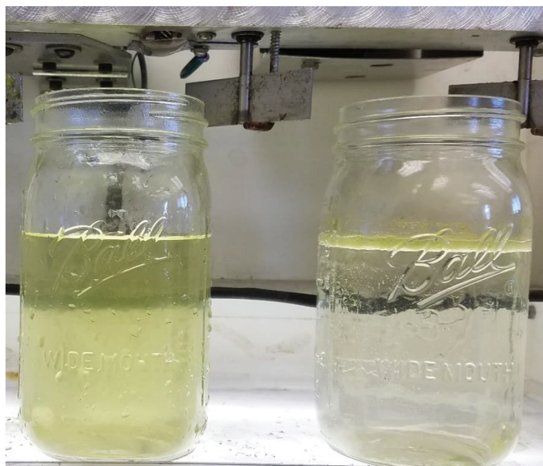
Samples taken from a facultative treatment facility. The left sample has not been treated and the right sample has been treated by the same methods as the Suspended Air® Flotation System but in a jar test environment.
